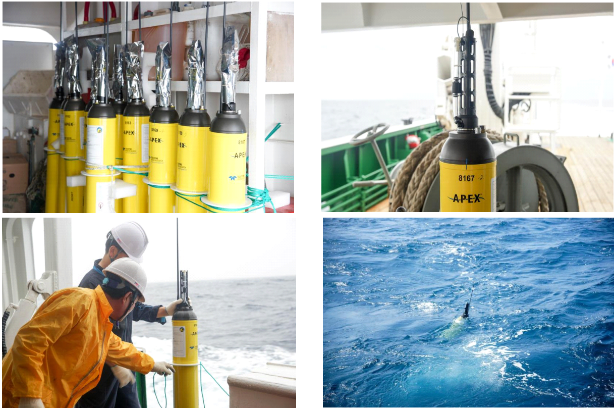
Fig.2. Several snap shots of the NIMS/KMA's Argo float deployment in 2017
